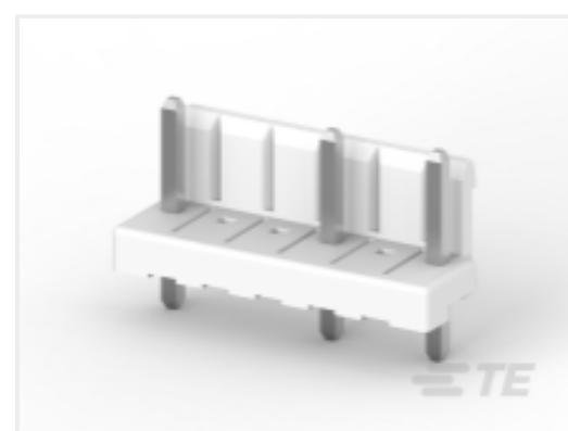
TE Part # 2316952-6 3.96 EP HDR ASSY 6P, NO PIN 2,3,5
