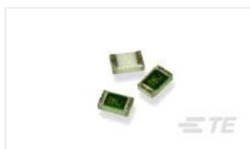
TE Part #9-1879208-9 CPF0402 150K 0.1% 25PPM 5K RL
