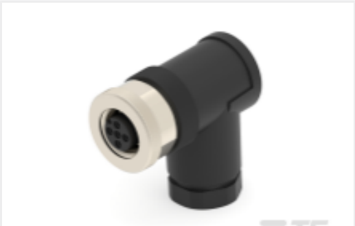
TE Part #T4112002041-000 M12,FEMALE,RA,A CODE,4P,PG9, GOLD
