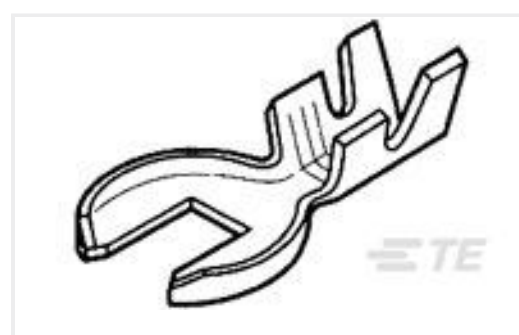
TE Part #60998-1 SPADE 16-14 AWG .0305 X .955 TPCU
