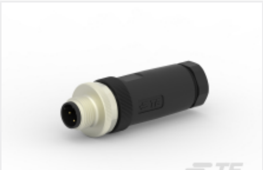
TE Part #T4111502041-000 M12,MALE,STRAIGHT,D CODE,4P, PG9,GOLD
