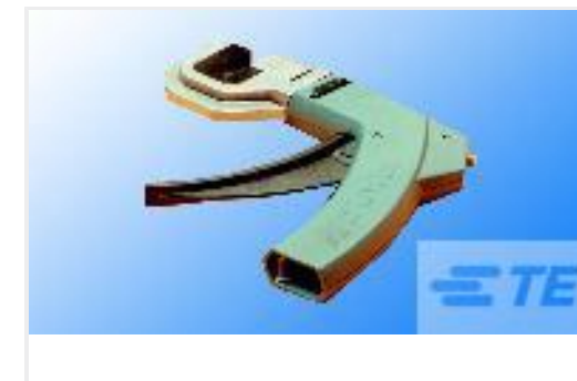
TE Part #58246-2 MTA 100 CRIMP HEAD PRODUCTION DISCRETE
