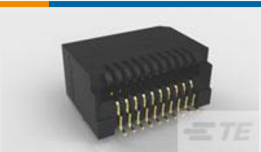
TE Part #1367073-2 20 POS SMT CONN, SFP, 30AU
