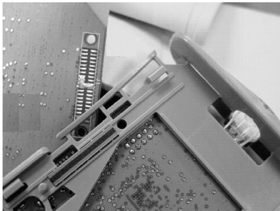
Dual-Row STAX Connector connects two rows of contact pads. Retention slot is provided in PCB separator.
