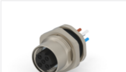
TE Part #T4171110505-001 M12,REAR MOUNTING,FEMALE,D,5P, 0.2M WIRE
