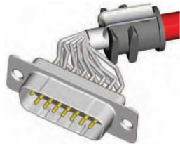
Bend cable shielding back on outside of strain relief
