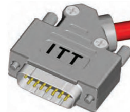
Assemble the other half (screwing force: 100-120 Ncm)
