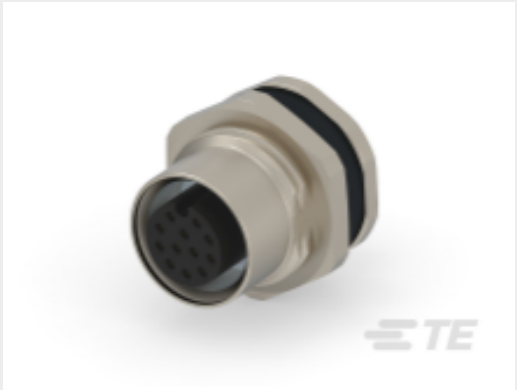
TE Part #T4171130012-001 M12,REAR MOUNT,FEMALE, A, 12P, 0.2M WIRE
