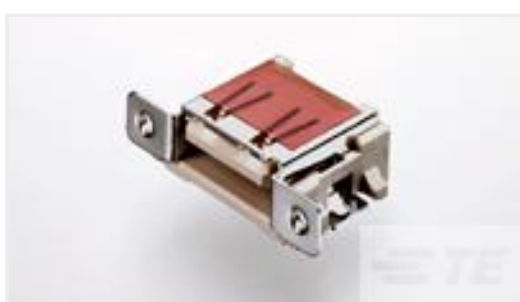
TE Part #5353928-1 Std USB Type A, R/A, SMT, Offset, Panel
