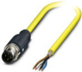
Sensor/Actuator cable, 4-position, PVC, yellow RAL 1021, shielded, Plug straight M12 SPEEDCON, A-coded, on free cable end, Cable length: 5 m
