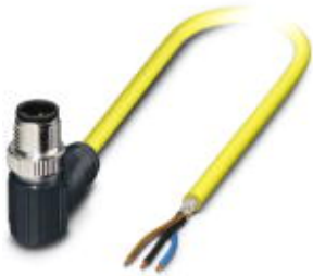
Sensor/Actuator cable, 3-position, PVC, yellow RAL 1021, shielded, Plug angled M12 SPEEDCON, A-coded, on free cable end, Cable length: 5 m
