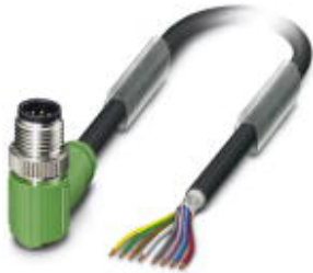
Sensor/actuator cable, 8-position, PUR halogen-free, black-gray RAL 7021, shielded, Plug angled M12, A-coded, on free cable end, cable length: 1.5 m
