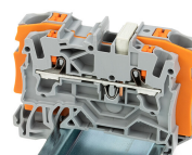
Step-down jumper (2006-499) commons 6/4 mm² (10/12 AWG) terminal blocks (2206/2204 Series) with 4/2.5/1.5 mm² (AWG 12/14/16) terminal blocks (2204/2202/2201 Series).
